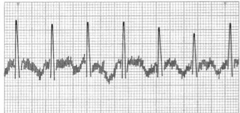
AC (60-cycle) interference
