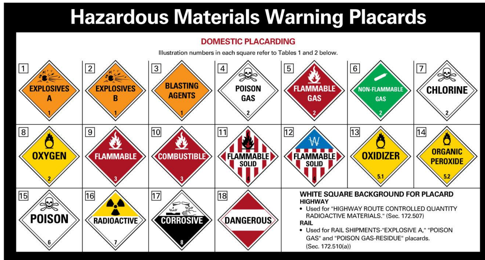
FIGURE 3-30B Transport Canada also requires display placards to be placed on the outside of vehicles.
